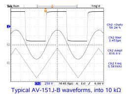
The AV-151 series is a family of high-voltage (or, for the AV-151F, high-current) function generators and variable-gain amplifiers. All models include both an internal oscillator that can generate sine, triangle, and square waves, and a variablegain amplifier mode, which permits generation of more complex high-voltage waveforms.
